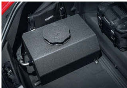
Reservoir holds water for the air-to-water intercoolers.
