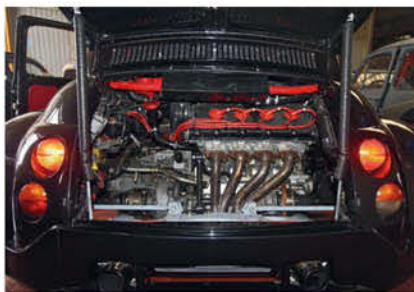
Installing the Ferrari V8 seems a relatively easy task compared to the V12...
