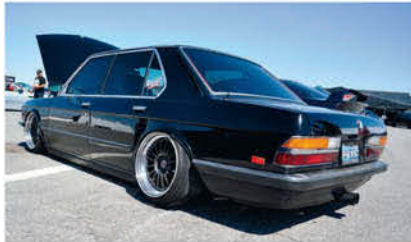
Sitting on airbags and fenders stuffed with HRE wheels, this E28 was motivated by a twin-turbo Supra engine and was also part of the Eurosquad Las Vegas posse.
